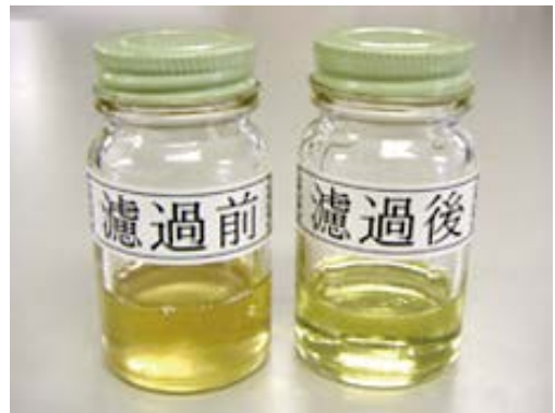
Color comparison before and after oil filtration
